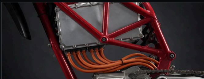
THE ELECTRIC HEART. BATTERY IN THE MAIN TRIANGLE; SIX ORANGE HV CABLES INTO THE MOTOR AT THE PIVOT.
