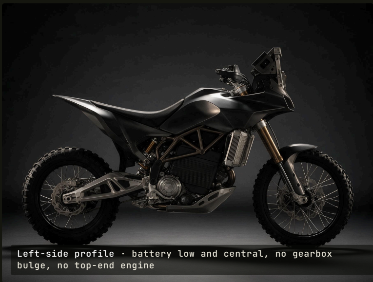
Exposed core • buffer pack in the trellis, axial-flux motor, twin rads
