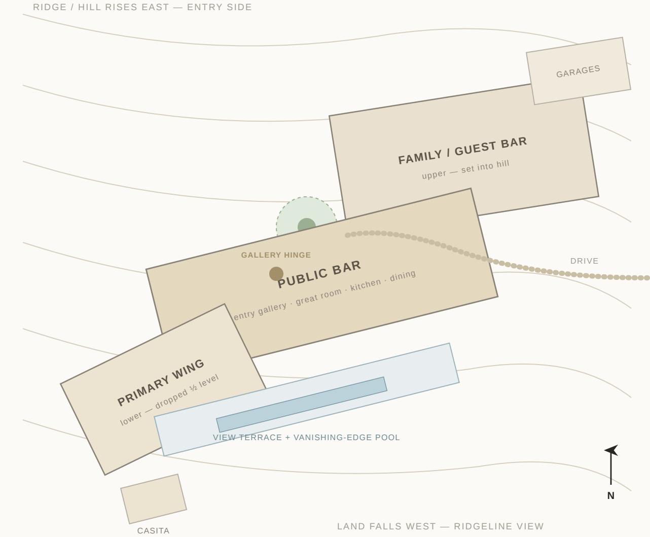
PARTI DIAGRAM — THREE BARS PINWHEEL AROUND THE ENTRY GALLERY, STEPPING DOWN THE SLOPE. NOT TO SCALE.
