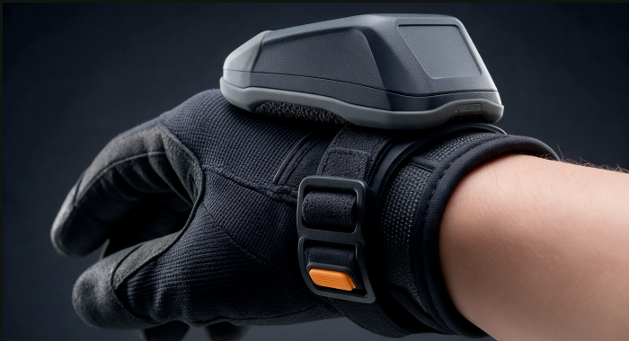
FIG. 05 Glove-over by default — the cam-and-hook-and-loop closure works by a gloved hand with no fine pinch; the amber pull-tab is the findable grab point. The mount is the cheap, laundryable, replaceable part.
