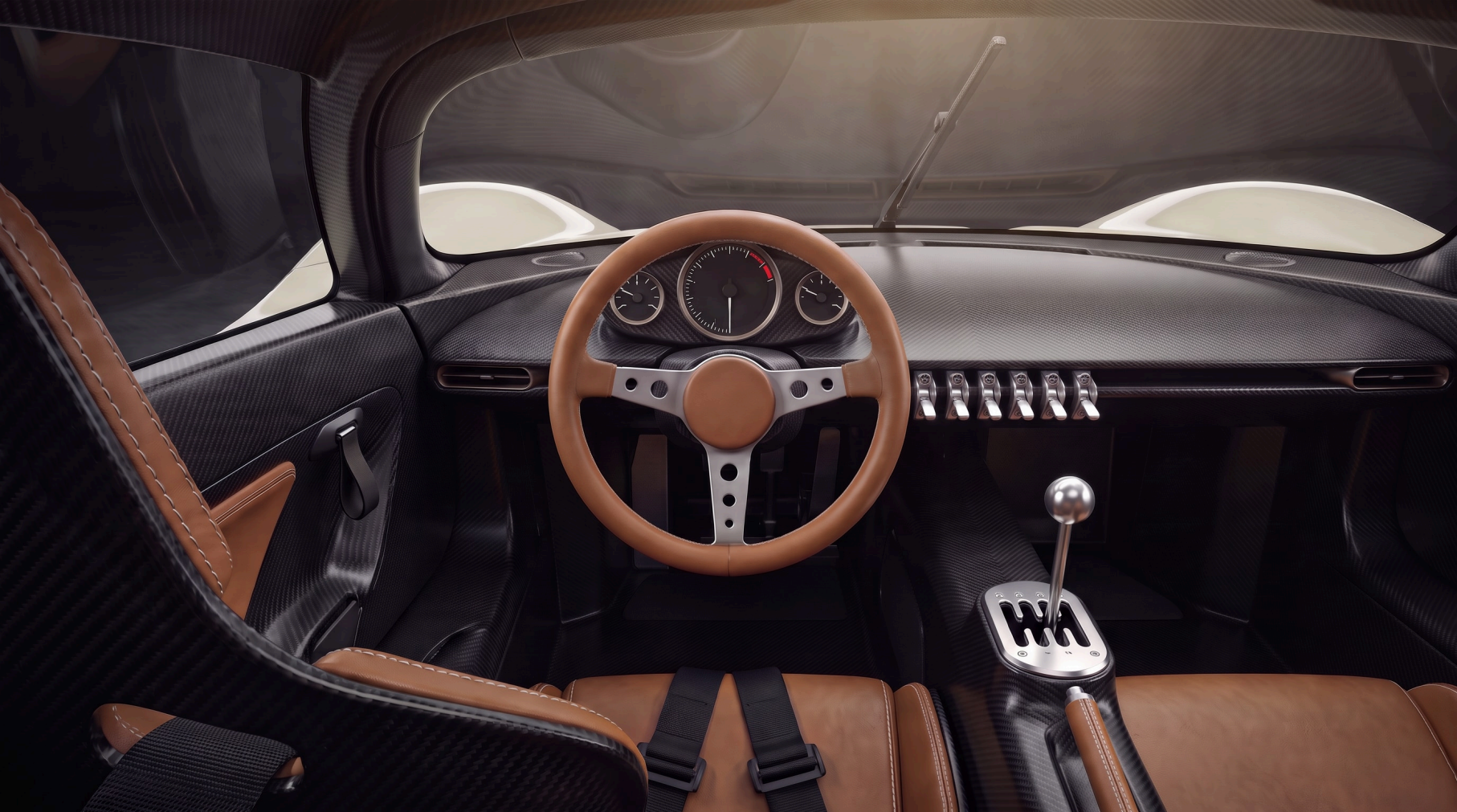
PLATE 5 The cockpit from just behind the driver's seat. Drilled three-spoke wheel, the oval binnacle and its three dials, six guarded toggles, the lever in its open gate.
