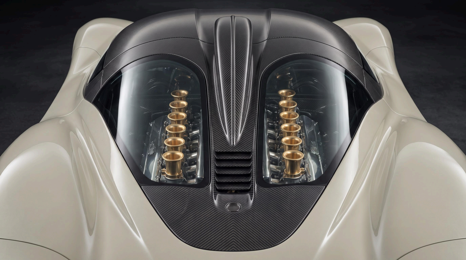
PLATE 2 The engine cover from above. Twelve gold-anodized stacks, six to a bank, under two glasses either side of the carbon spine fin and its louvers.
